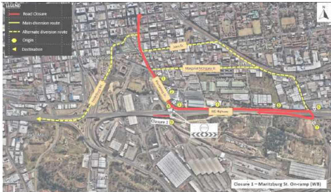
Figure 2: Diversion Route for Maritzburg St. On-ramp
